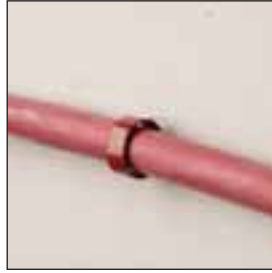
It takes 107 N (24 lbs) average force to pull out the clip.
