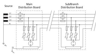
\* Install fuse A if supply fuse B exceeds back-up overcurrent protection rating
