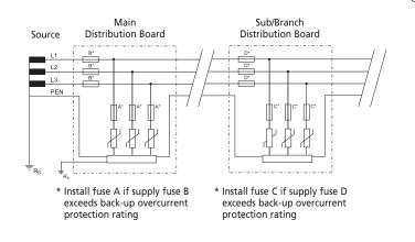
require SPD s to be installed in all the modes detailed. The following diagrams provide guidance on the selection and installation of SPDs on the more common distribution systems. While three phase WYE systems are shown, similar logic can be applied to single phase, delta and other configuration sources.
