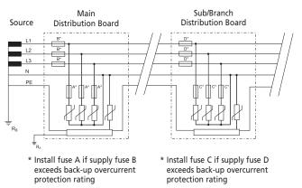
SPDs shown connected L-N and N-PE. May also be connected L-PE and N-PE.
