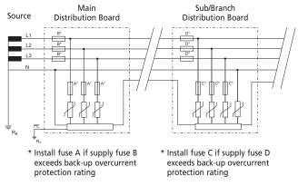
SPDs shown connected L-PE and N-PE. May also be connected L-N and N-PE.
