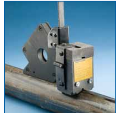
"A" Price Key Mold on Steel Pipe
