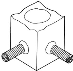
**ANSWER:** NO! Neither mud nor anything else containing water or oil should ever be used. CADWELD **T403** Mold Sealer packed around the conductors AFTER the mold handles have been closed and locked will usually stop the leakage. However, after the mold wears and the cable opening becomes enlarged, the difference between the mold opening and the cable diameter may be too great for the mold sealer to do its job. A new mold will then be required.
