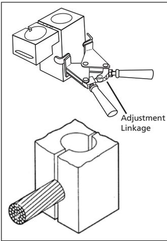
**ANSWER 11a:** The first thing to check is the adjustment of the handles, especially if the handles are new. Just in front of the grips is the adjustment linkage. Remove the key and pin. Turn the linkage counterclockwise to tighten the locking action and clockwise to loosen the locking action. Test the locking action and then replace the pin and key.
