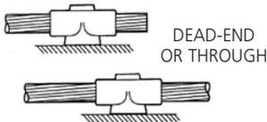
**ANSWER 3f:** When making connections of vertical cable to a vertical steel surface, a **Type VV** mold can be used for a through cable, a dead-end cable from above or a dead-end cable from below.
