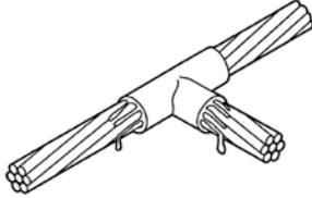
**ANSWER:** This is a common occurrence, especially after the mold has been used 15 to 20 times and the cable mold openings become worn. After the mold has been locked on the cables, apply a ring of CADWELD **T403** Mold Sealer around the cable where it enters the mold. Don't force it into the mold! If it gets in the weld cavity, the molten metal will cause it to burn and give off gases which can cause an improper weld or spattering of molten welding material.
