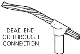
**ANSWER 3c:** For ground rods, use **Type GT** through cable connections. When the cable dead-ends at the ground rod, just let it extend past the rod 2" (through the mold) when making the connection.
