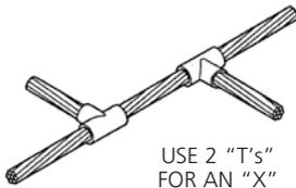
**ANSWER 3d:** When a lot of "T's" and a few "X's" are required on a job, use two "T's" about 2" apart to make the "X".
