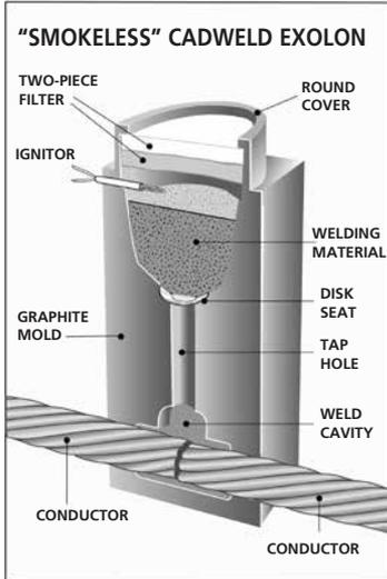
**ANSWER:** To deal with such situations, Pentair developed the CADWELD EXOLON low-emission welding process. The CADWELD EXOLON system produces the same permanent, highly reliable welded bonds as the standard CADWELD process, but without the smoke usually associated with the exothermic welding process.
