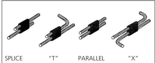
**ANSWER 3b:** When a splice is required, several different mold types may be used. For instance, a splice can be made using the same mold as other connections like a **Type TA**. Just center the ends of the cable to be spliced under the tap hole of the mold and use a short length of cable (about 3 inches) in the tap cable hole. Be careful to center the cable ends for the splice in the center of the mold.
