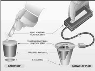
**ANSWER:** Pentair has developed a patented system that initiates the CADWELD reaction by delivering a specific amount of energy to the welding material using an ignition strip. The strip is constructed of metals and insulation. It is not flammable and cannot spark unless the Control Unit is attached and operated. One of the unique features of this system is that it has the capability of providing a second spark to initiate the reaction if necessary.
