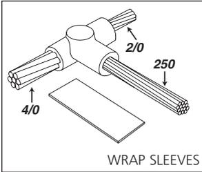
**ANSWER 1a:** You can often shim one or two cable sizes to fit a larger mold. Use a wrap sleeve, CADWELD Part No. **B140A**. Wrap the shim around each cable to build it up to a 4/0 size. Then use the 4/0 molds to make the connection. We recommend that you keep a package of wrap sleeves handy.
